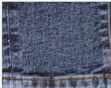
Conventional stonewash Liquor ratio 1:6 Stones 1:2 1.0 % Cellulase
