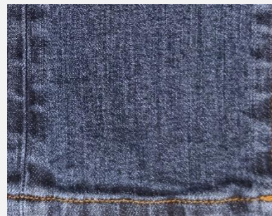
Enzyme treatment by fog Wetting degree 30 % 0.9 % organIQ BIOPOWER
